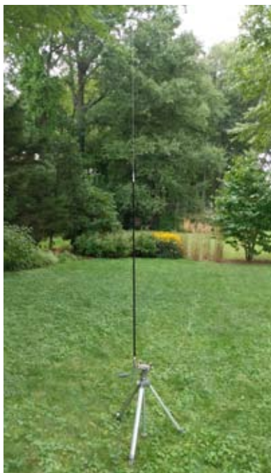
Hamstick on Tripod and Clamp Mounts with push-on counterpoise wire connections
