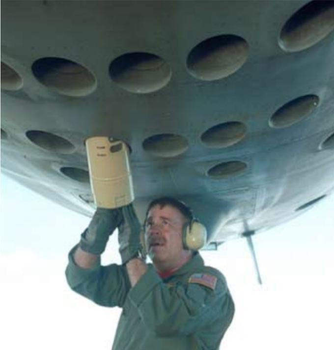
Loading Sonobuoy into Launcher on P-3 Orion
